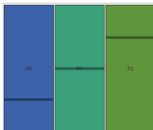
figure 37 - A screen of the processor display for three processors with an utilisation of 25%, 50% and 75% respectively all executing different actors.
